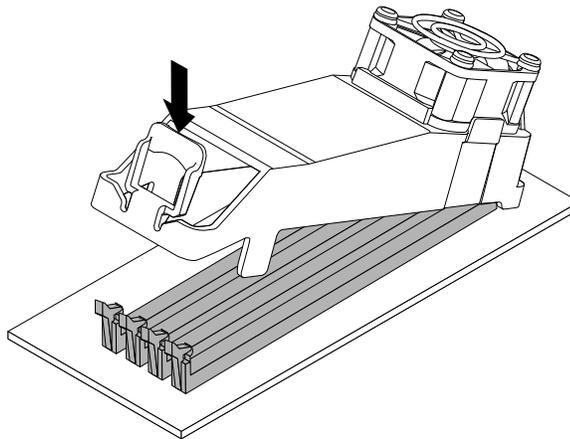
Figure 15. Installing the memory cooler
