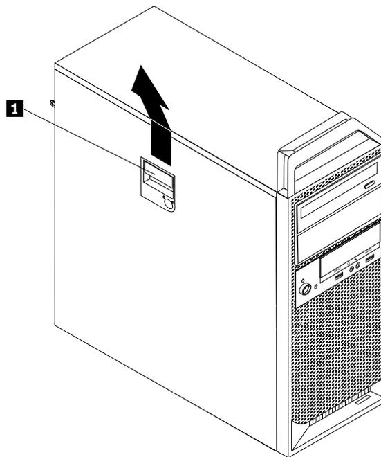
Figure 6. Removing the computer cover
