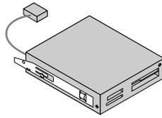
*Figure 21. Installing the card reader retainer*
