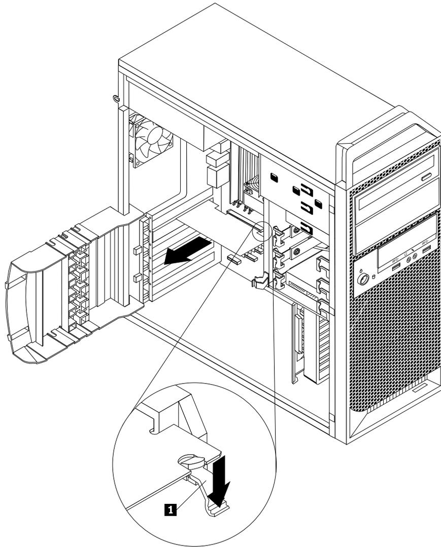
*Figure 9. Removing a PCI card*
