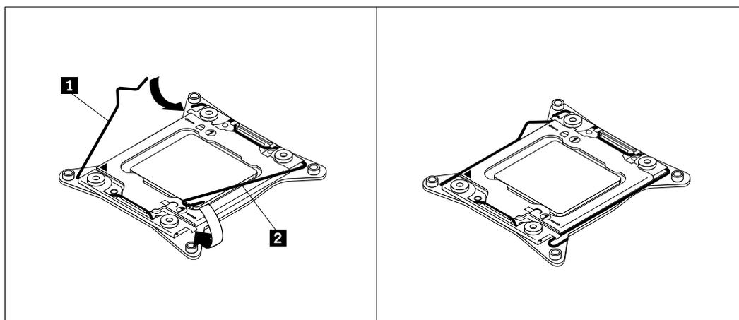
Figure 44. Securing the microprocessor in the socket
