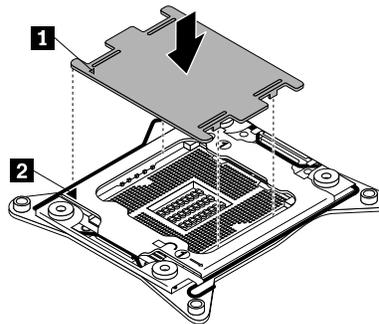
Figure 49. Installing the microprocessor socket cover
