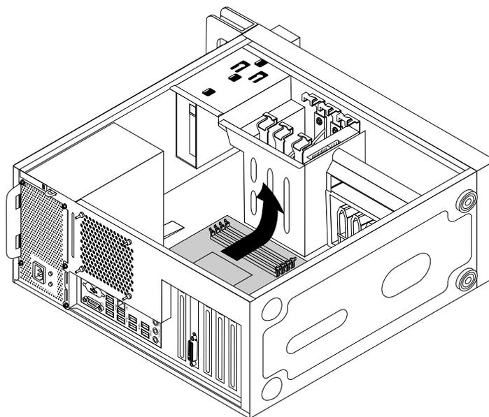
Figure 46. Removing the system board
