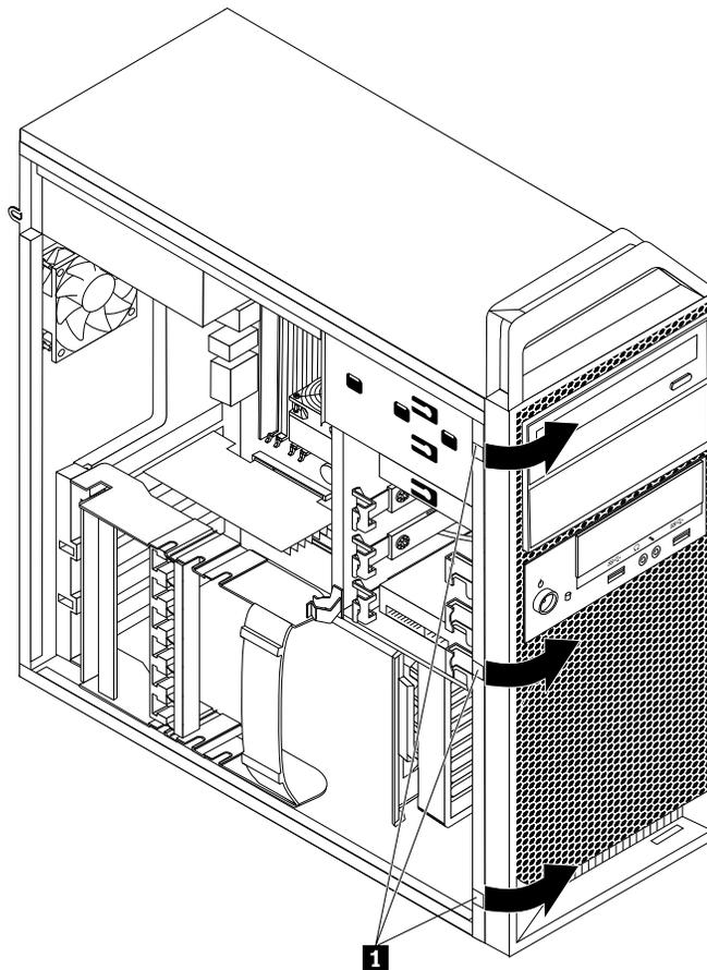
Figure 7. Removing the front bezel
