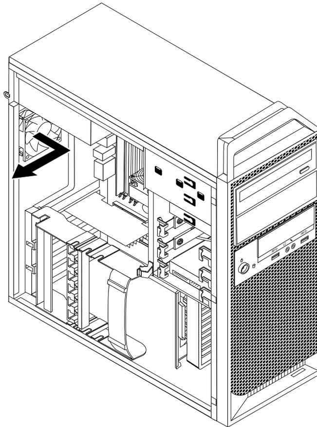
Figure 26. Removing the rear fan assembly
