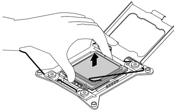
Figure 40. Removing the microprocessor
