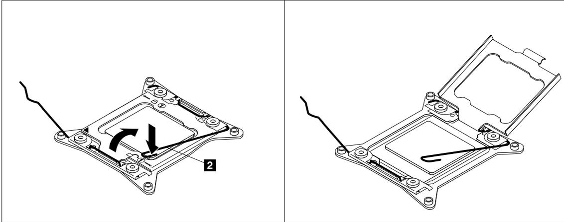
Figure 39. Opening the microprocessor retainer
