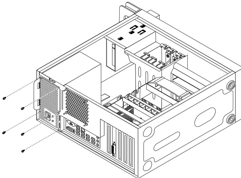
Figure 50. Removing the screws for the power supply assembly
