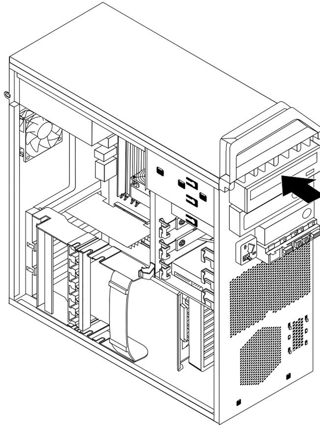
Figure 18. Installing the optical drive
