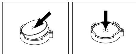
Figure 24. Installing a new battery
