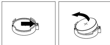
Figure 23. Removing the old battery
