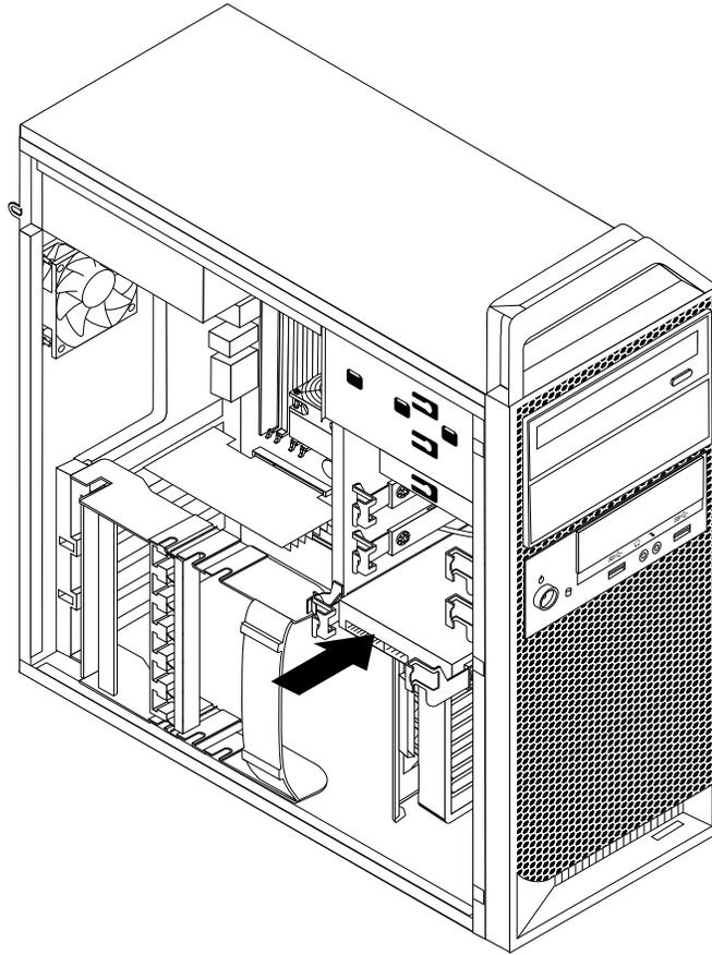
Figure 31. Installing a hard disk drive
