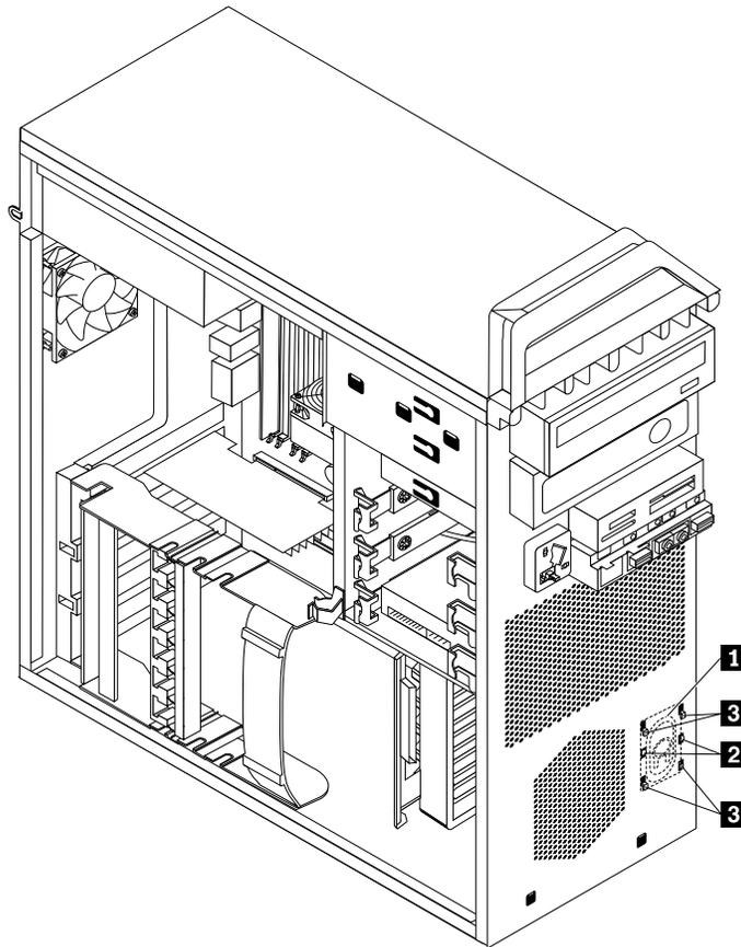
Figure 37. Removing the internal speaker
