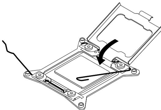
Figure 43. Closing the microprocessor retainer
