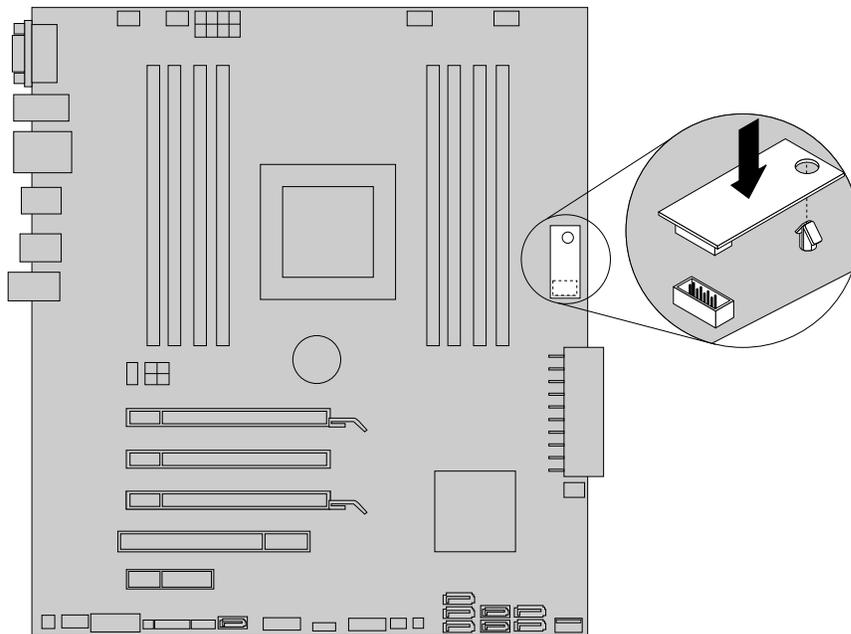
Figure 35. Installing a new hard disk drive enablement module
