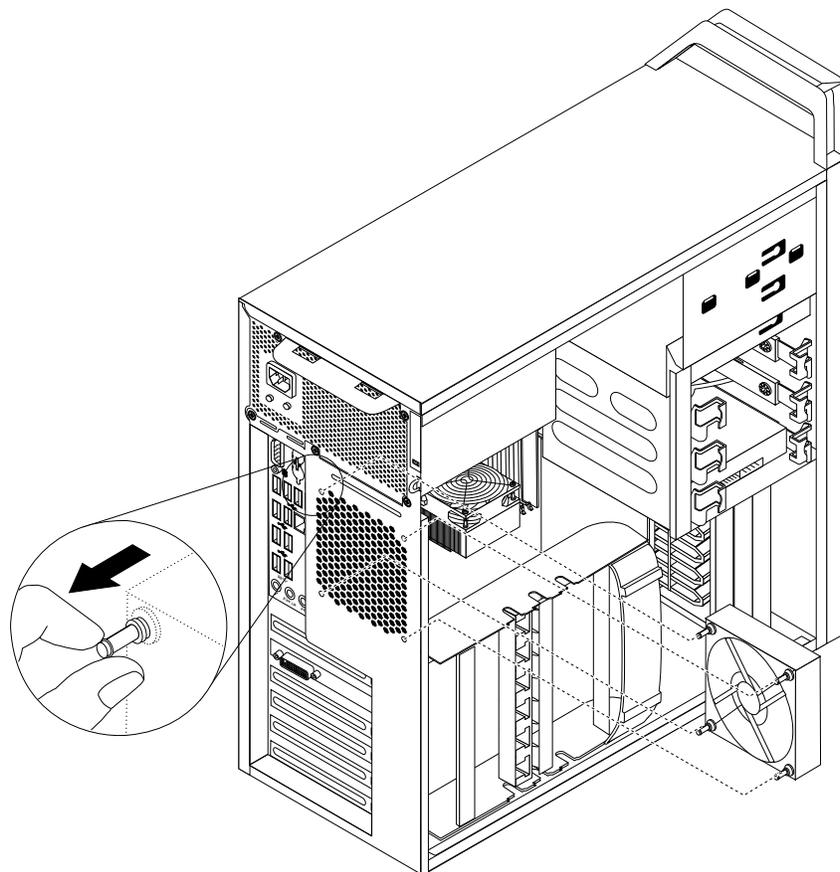
Figure 27. Installing the rear fan assembly
