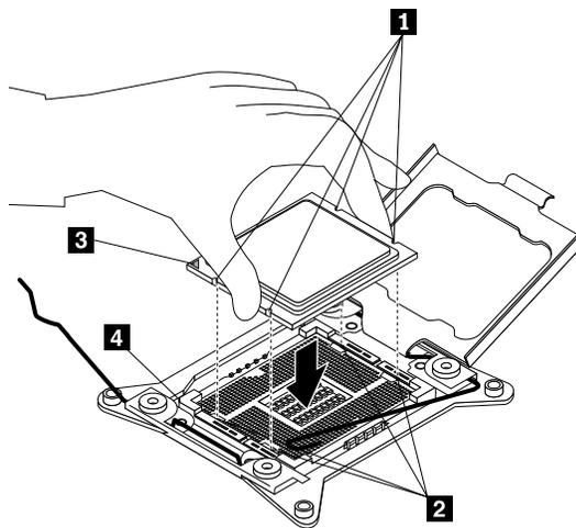
Figure 42. Installing the microprocessor
