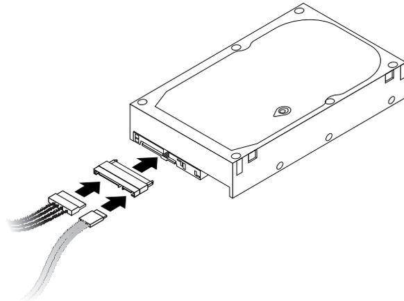
Figure 33. Connecting a SAS hard disk drive
