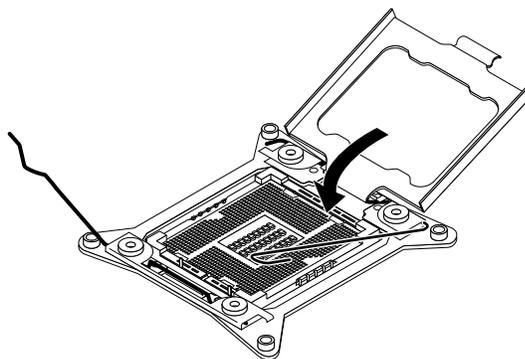
Figure 47. Closing the microprocessor retainer
