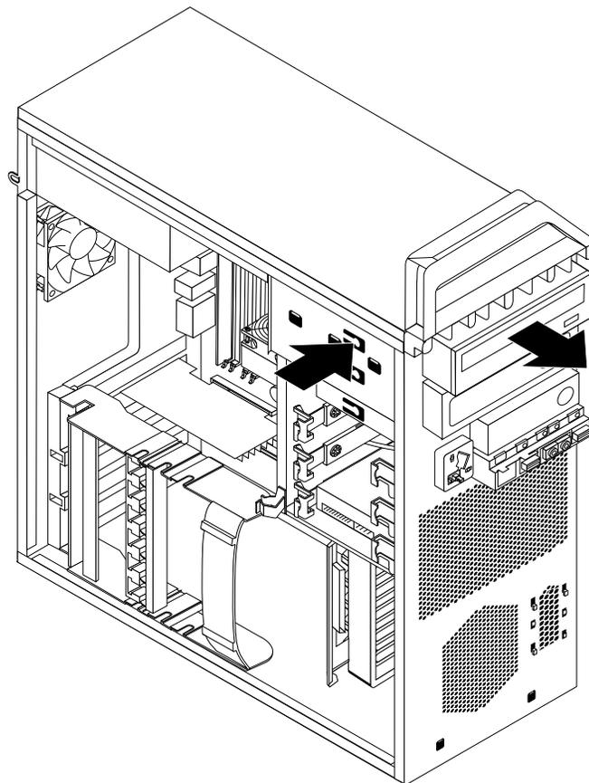
Figure 16. Removing the optical drive
