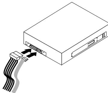
Figure 19. Connecting the optical drive
