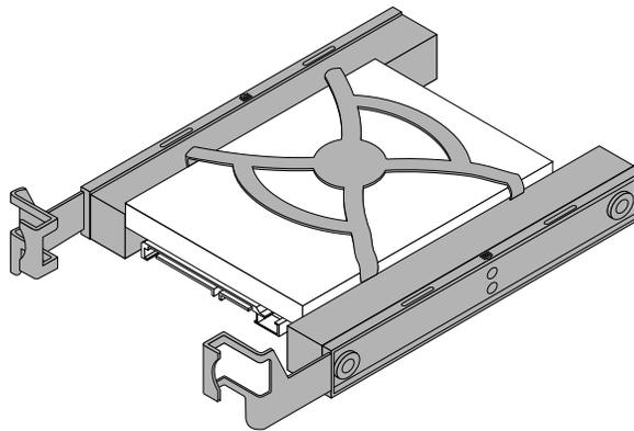
Figure 30. Installing a 2.5-inch hard disk drive into the bracket
