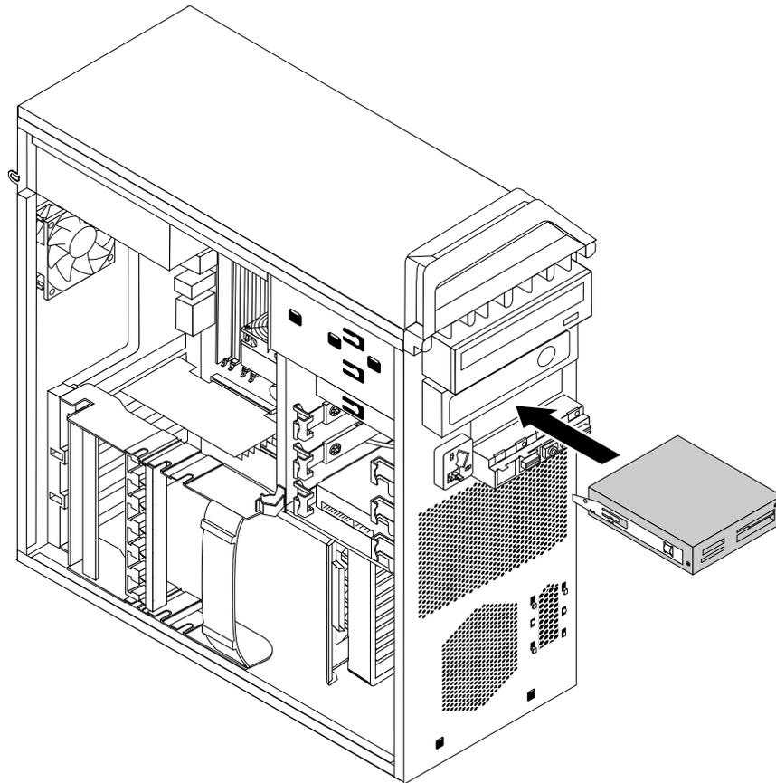
*Figure 22. Installing the card reader*
