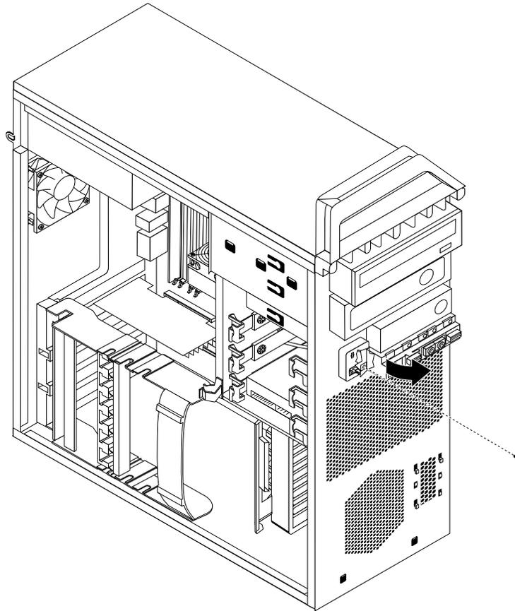
Figure 36. Removing the front audio and USB assembly
