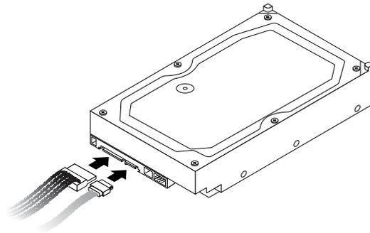
Figure 32. Connecting a SATA hard disk drive
