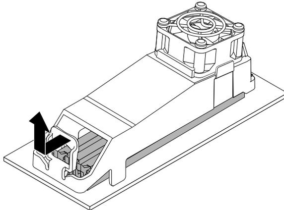
Figure 11. Removing the memory cooler
