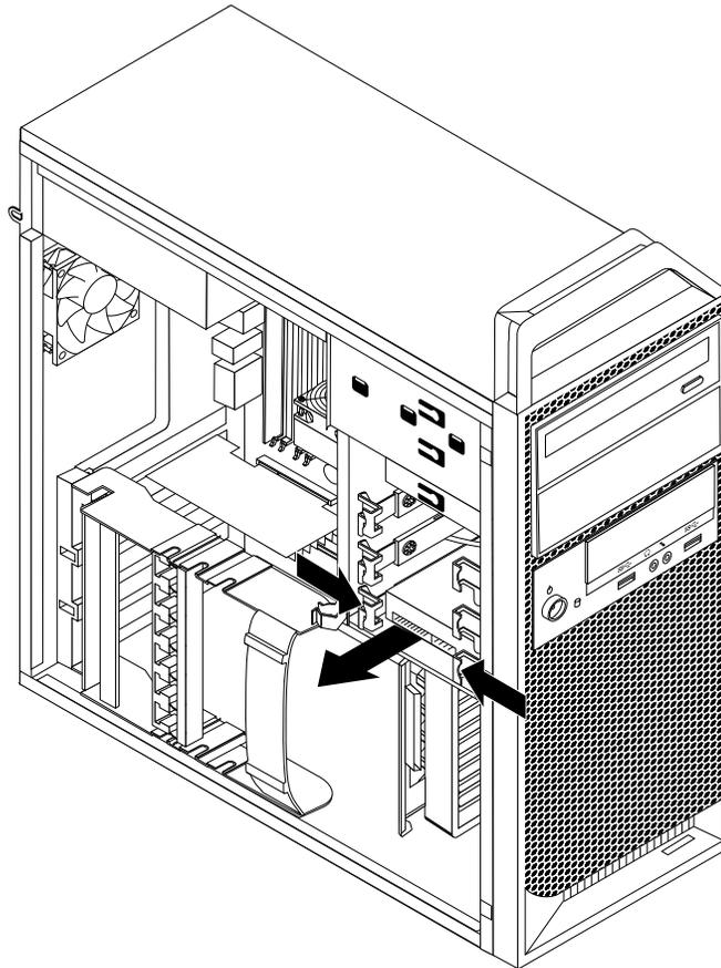
*Figure 28. Removing a hard disk drive*
