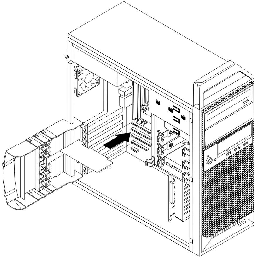
Figure 10. Installing a PCI card
