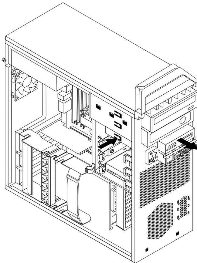
Figure 20. Removing the card reader
